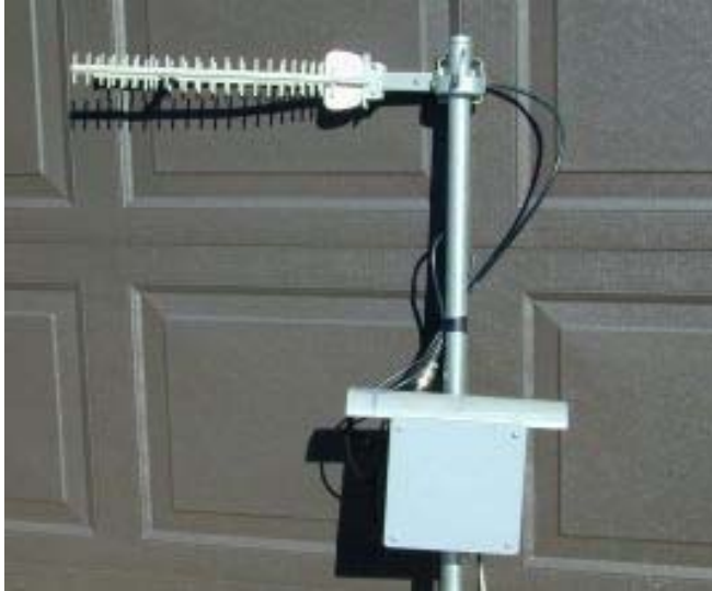
Figure 2-8: Enclosing a Bridge within a NEMA Box
