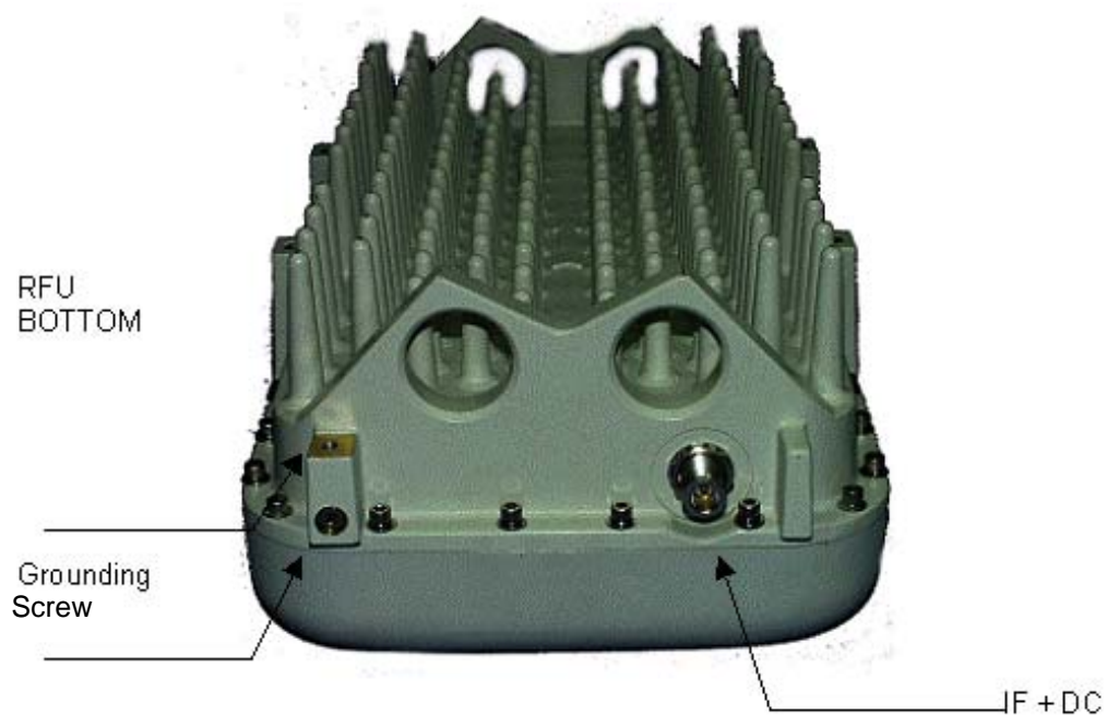
Figure B-2: Alvarion WALKair ODU Grounding Point
