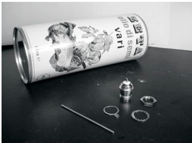
Figure 4.34: Parts needed for the can antenna.
