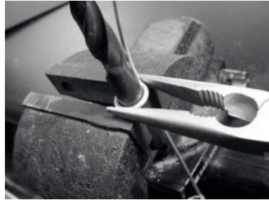
Figure 4.18: Bend the wire around the drill bit to make a coil.
