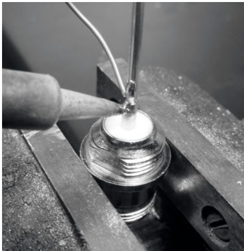
Figure 4.39: Solder the wire to the gold cup on the N connector.
