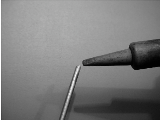
Figure 4.38: Tin the end of the wire before soldering.
