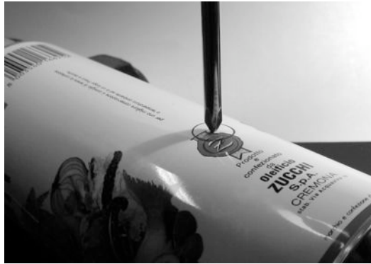
Figure 4.36: Mark the hole before drilling.
