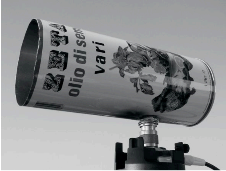
Figure 4.33: The finished antenna.
